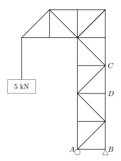
In kN, what is the force experienced by the rod CD? Express a positive number if the member is in tension and a negative number if it is in compression.
