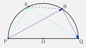
We define angles as  $\angle APB = \angle AQB = \gamma$ ,  $\angle AOB = 2\gamma$ ,  $\angle BPQ = \alpha$ ,  $\angle AQP = \beta$ . Note that  $\overrightarrow{PA} = I_2 \omega L$ ,  $\overrightarrow{AQ} = I_2 R$ ,  $\overrightarrow{PB} = I_1 R_1$ ,  $\overrightarrow{BQ} = 1/I_1 \omega C$ . We seek to maximize the length of AB. We can write via law of cosines that
