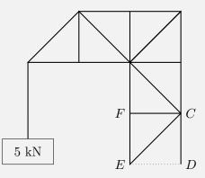
Since the net force of this sub-element is still zero, we can do a force balance. The only *external* forces acting on this system is EF, EC, CD, and the 5kN weight. If we do a torque balance about E, we get:
